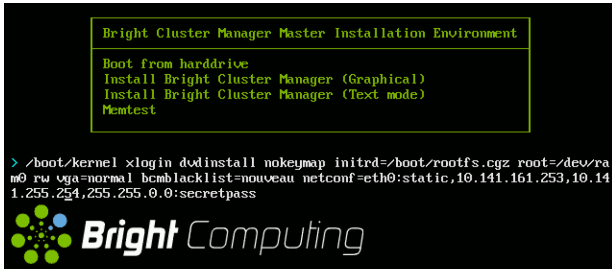
Figure 3.1: Installation: ISO Boot Menu For Legacy BIOS
